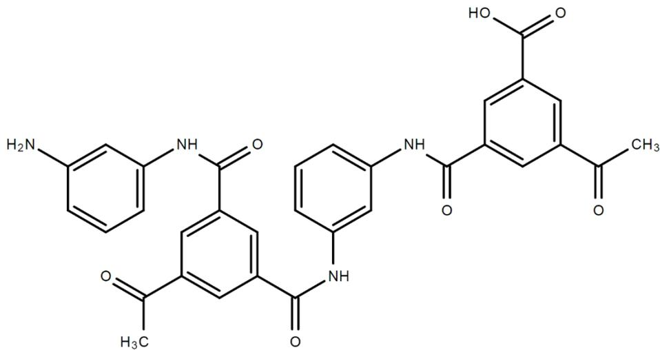
**Figure 3.** The approximate structure of the aromatic polyamide membrane.
