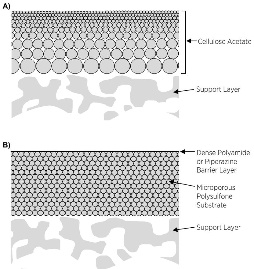
**Figure 2.** Cross sections of **A)** cellulose acetate membranes and **B)** thin-film composite membranes.
